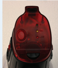
Whistle button, adjustable volume, and battery indicator
