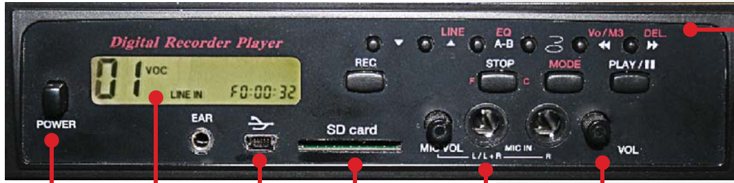
POWER LCD SCREEN USB SD CARD SLOT MIC CONTROLS MASTER VOLUME RECORDING CONTROLS
