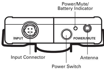
**Figure G-Handheld Transmitter Bottom View**
