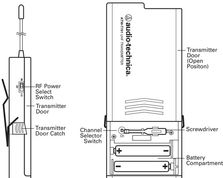
**Handheld Transmitter Battery Installation**
