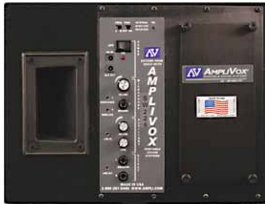
Back of SW225: amplifier control panel
